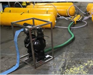
Aluminium Air Powered Diaphragm Pump in Metal Frame Pump Air Hose
