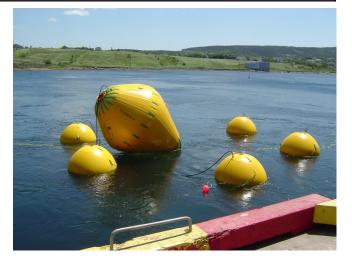
Enclosed Parachute design for stable use in currents and during re-floatation, low speed towing and positioning.
